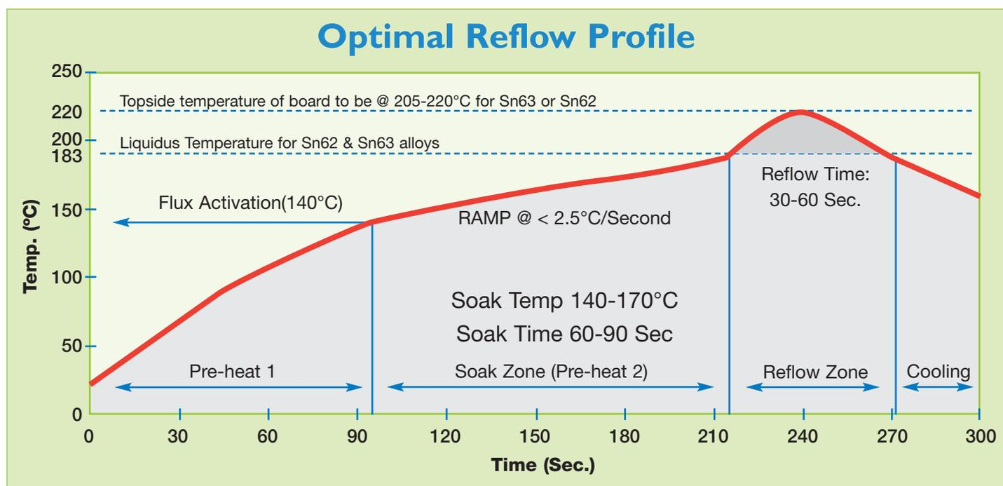
Many reflow machines available today include an on-board profiler, even some of the smaller, less expensive, bench-top ovens. If the oven being used is not equipped with a profiler, after market temperature profilers are available.
