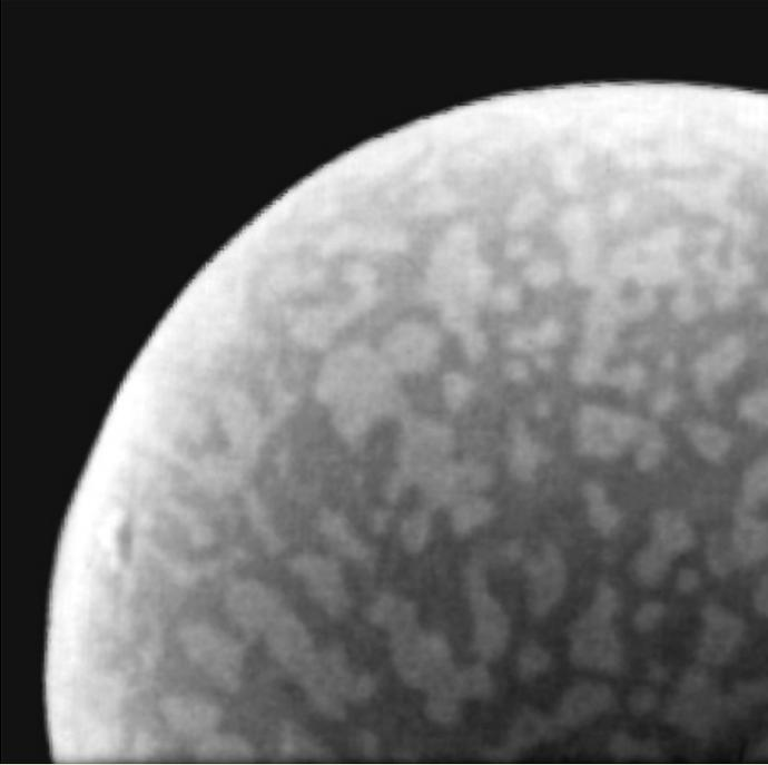
*62Sn/36Pb/Ag<sub>2</sub> solder powder particle enlarged from 1000x scanning electron micrograph.*
