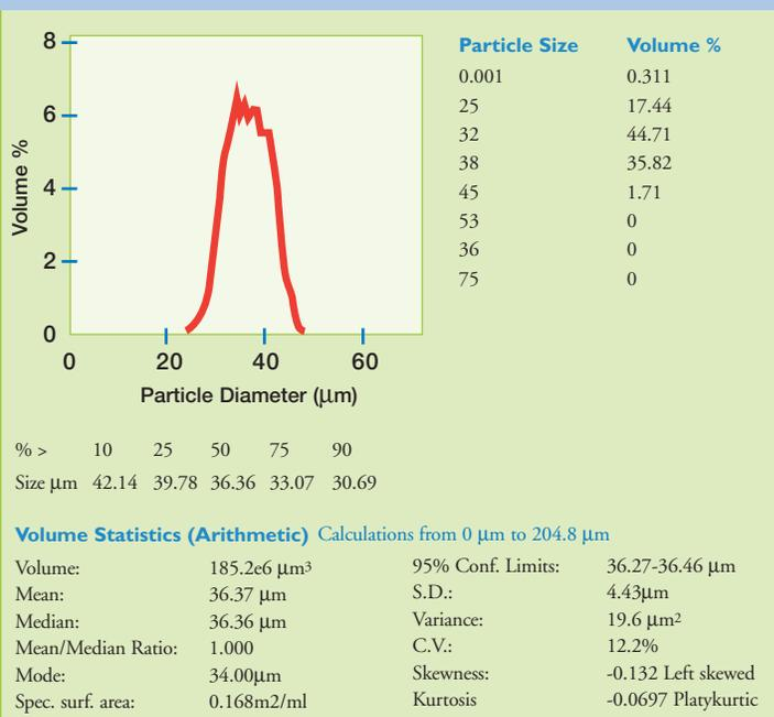
Therefore, to properly specify a powder, it is necessary to recognize that it is a population of particles, and it is necessary to characterize that population in terms of the distribution of parameters that are important to the particular application.
